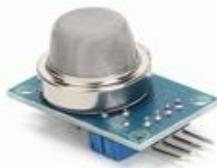
Gambar 4. Sensor Gas MQ-6
