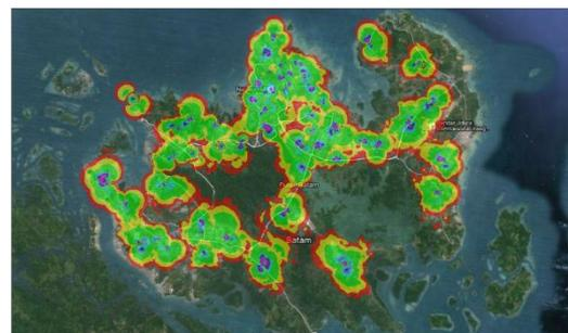
Gambar 9. Uplink Throughput 20 MHz FDD
