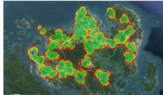
Gambar 7. Uplink Throughput 10 MHz FDD
