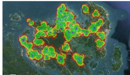
Gambar 8. Uplink Throughput 15 MHz FDD
